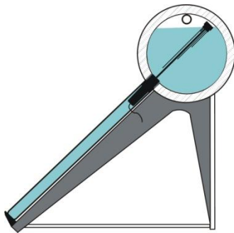
Sensor installed on the bottom collector tube hole
