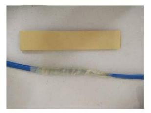
4 Cover the whole cable with the big heat shrinkable tube
