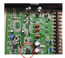
Here are three positions for the SOLAR-BAT diverter switch: solar array position, power-stop position(middle) and battery position. When using the solar array and battery, you only need to turn this switch to change the battery mode and solar mode.
