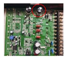
If you turn the speed button counterclockwise all the way, the system efficiency will decrease to only 30% of original efficiency. When turn the speed button clockwise\_all the way, the system efficiency will be 100%.
