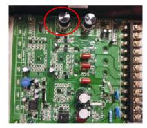
Turn the Time delay button to the constant number (the engraved lines at the top of button to the constant number). If the system checks that the well water level is lower than the water level sensor, the system will stop working and the WELL indication light will be on. When the well water level is higher than the water level sensor, the WELL indication light will start to blink until the delay time is over and WELL indication light is off and the system start to work.
