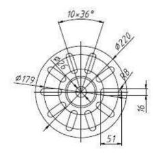
Flange diameter as 200mm, with 8slots
